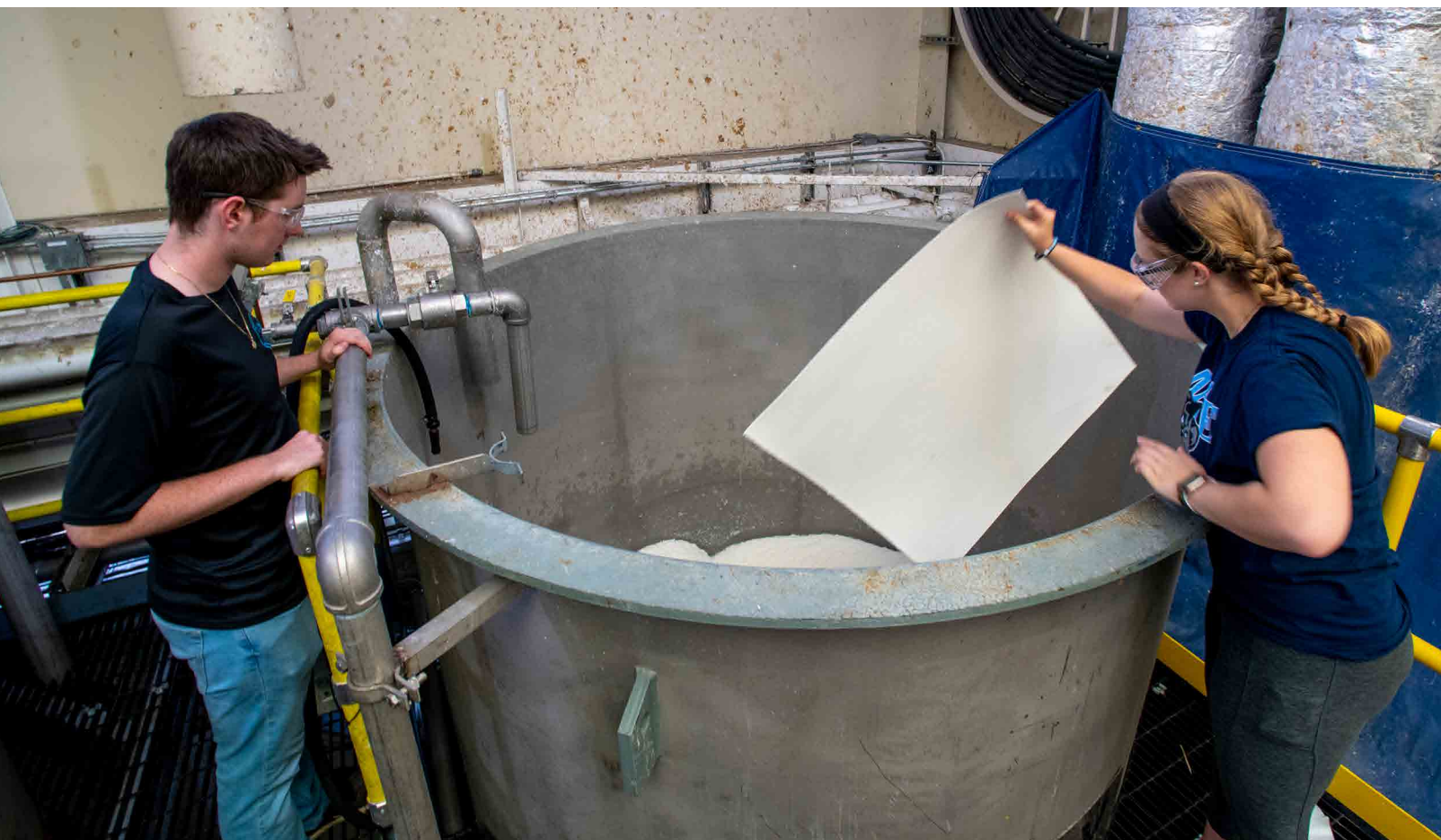
UMaine nanocellulose production in the Process Development Center begins with rehydrating sheets made from wood pulp.
