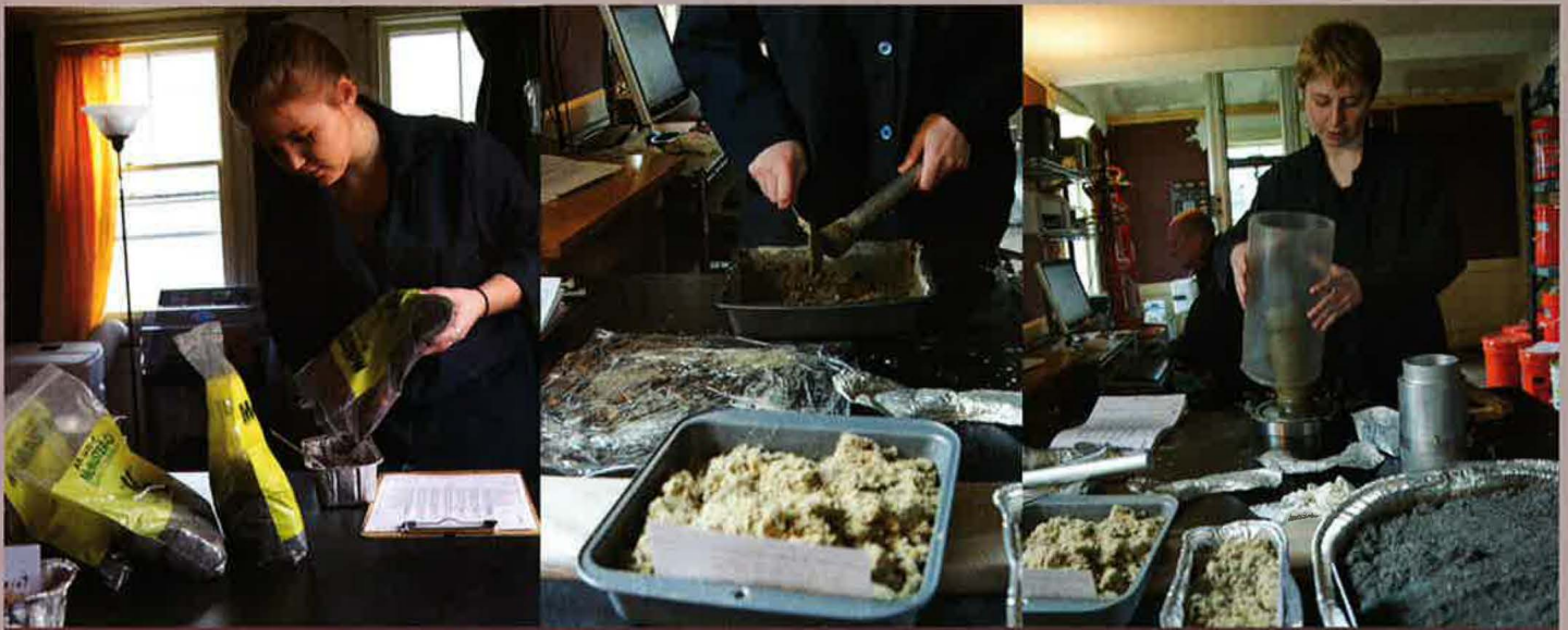
In the Racing Surfaces Testing Laboratory, UMaine undergraduate Julia Bradson, left, prepares samples from racetrack surfaces for the drying ovens. In preparation for triaxial shear testing, Molly Segee then mixes the dried material with a measured amount of water and compacts it.
