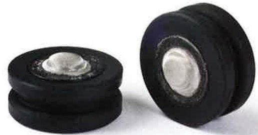
The OSS swabs work like a "nanosponge" that interfaces directly with a portable, computerized, infrared spectrometer made by Smiths Detection.
