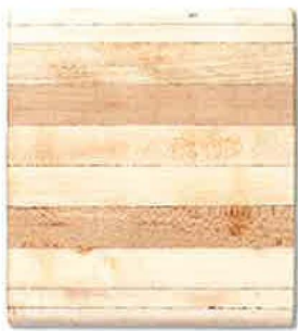
Advanced Engineered Lumber (AEL) is a new beam and column composite product developed by UMaine's Advanced Engineered Wood Composites Center. Now, Engineered Materials of Maine will manufacture AEL from layers of solid, low-grade sawn hardwood up to 1.5 inches thick.
