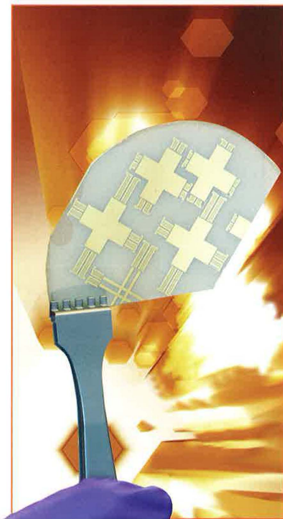
Surface acoustic wave devices, which will serve as fluid transport and processing components of the endospore detection microsystem, are fabricated through a thin film photolithographic process using a piezoelectric substrate.
