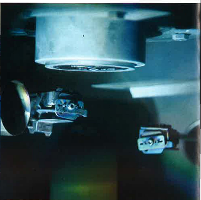
LASST research scientists George Bernhardt, left, and David Frankel prepare to deposit thin film coatings on the sensor devices. The photo on the right shows the film deposition configuration inside a vacuum chamber. In the top photo, a prototype sensor is tested over the long term in a high-temperature furnace at LASST.
