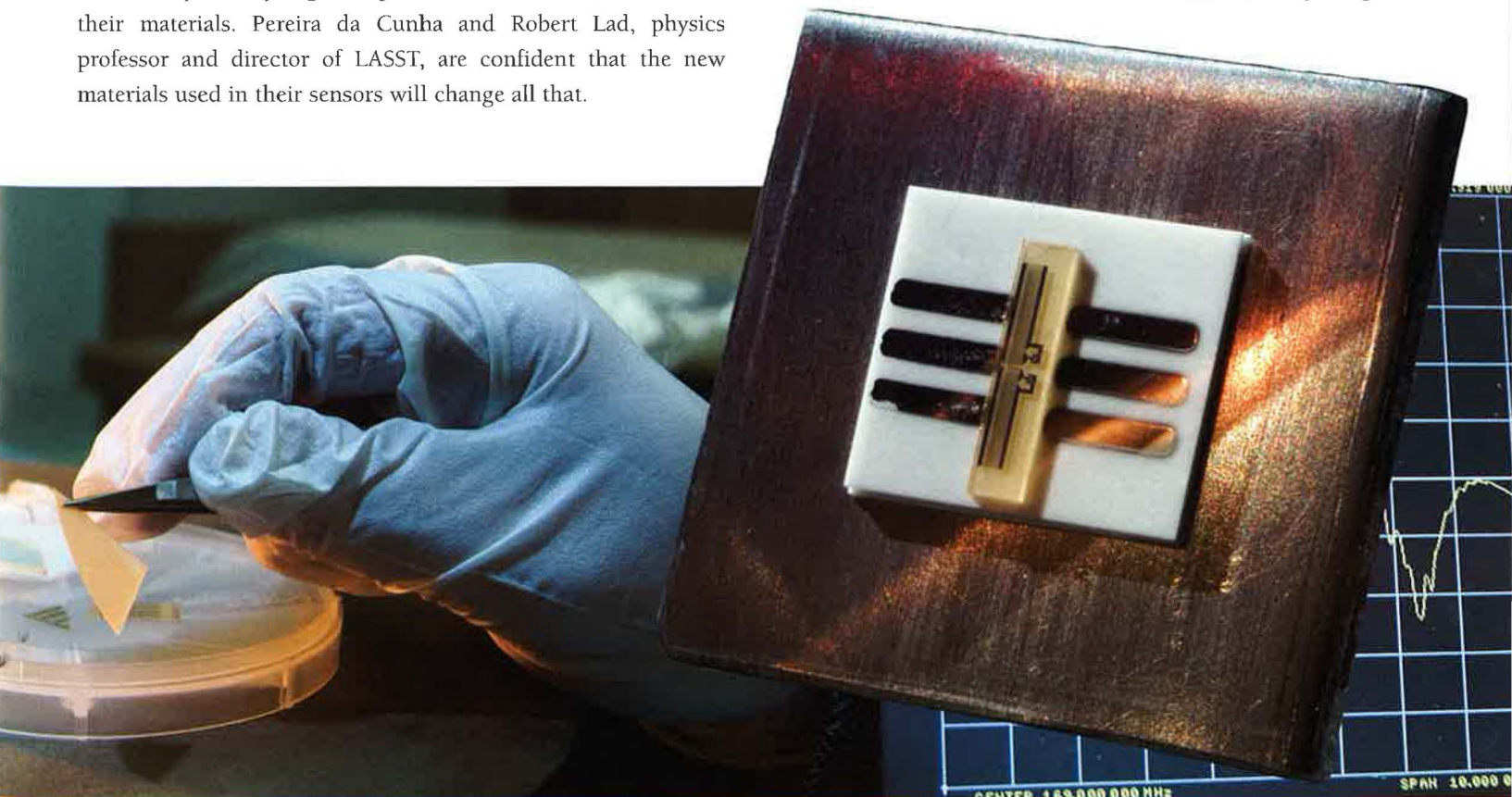
The acoustic wave sensors, like the one pictured above, right, are made using a crystalline material called langasite that is cut into wafers just 500 microns thick. To further enhance the sensor's high-temperature capabilities, ultrathin ceramic film materials have been developed to coat the device.
