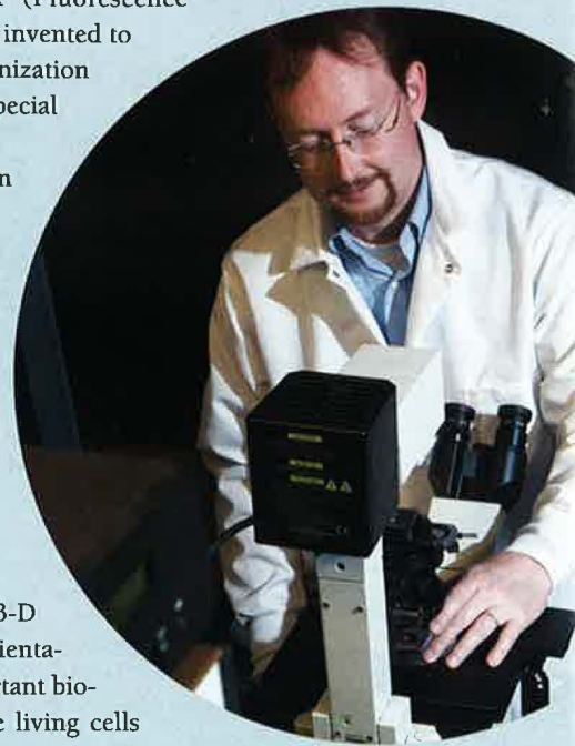
The FPALM microscopy system breaks a fundamental limit on the resolution of lens-based microscopes, known as the diffraction barrier, which has existed for more than 100 years.
