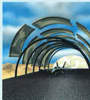
Inflatable arches provide structural support for a portable hanger. Illustration by Knife Edge Products
