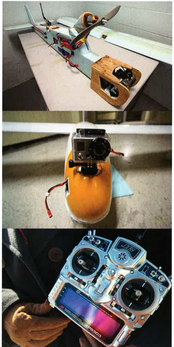
Top photo: Brian Barainca also built Blue, Gannet's companion, to test equipment. A waterproof and shockproof GoPro camera perched atop Gannet's nose provides a bird's-eye view of land, sea, sky and birds. The operator controls Gannet's takeoffs, altitude, speed, loops and landings with a hand-held transmitter.
