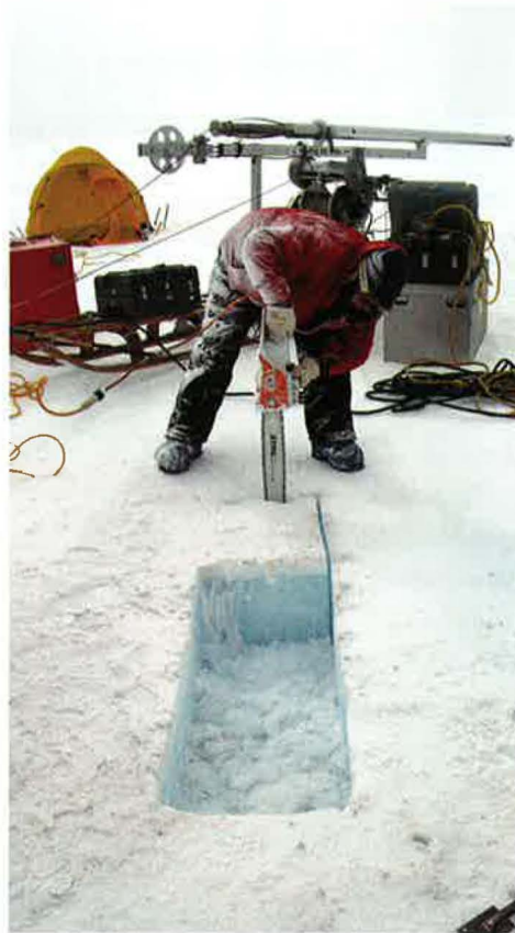
In the Blue Ice Area, a horizontal trench is cut to sample large volumes of ice from the surface.
