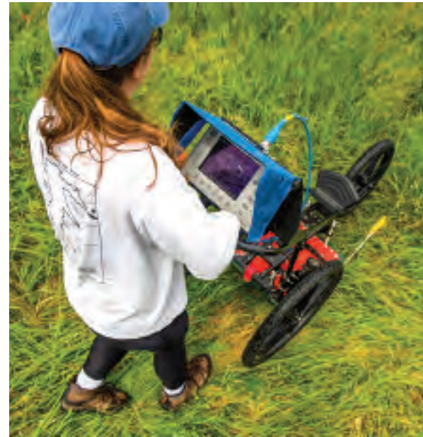
Ground penetrating radar (GPR) uses short radar pulses to discover and identify features beneath the ground surface.
