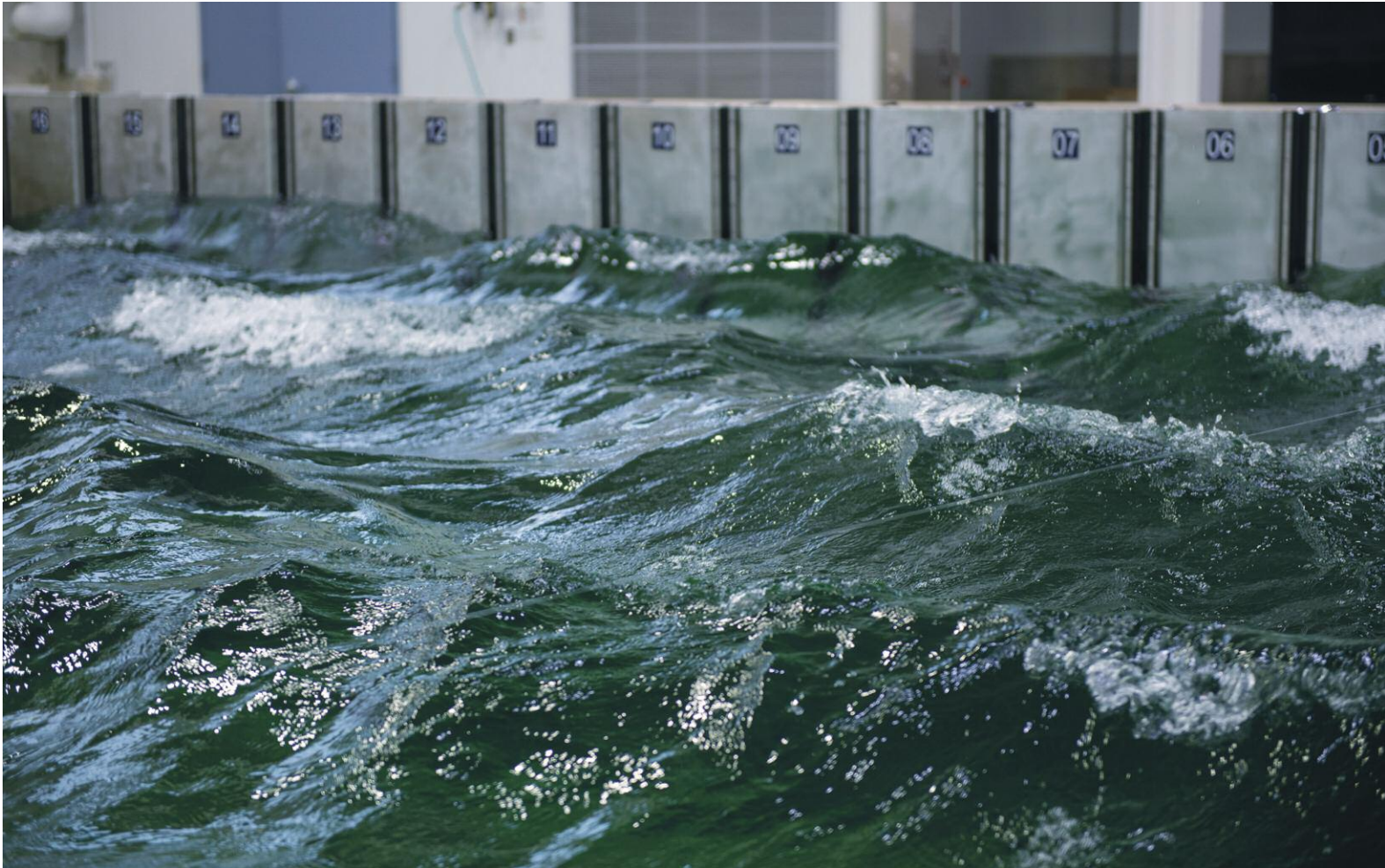
The wave maker at one end of the basin is capable of creating waves of varying frequency and as high as 0.8 meters (equivalent to 40 meters at full scale).
