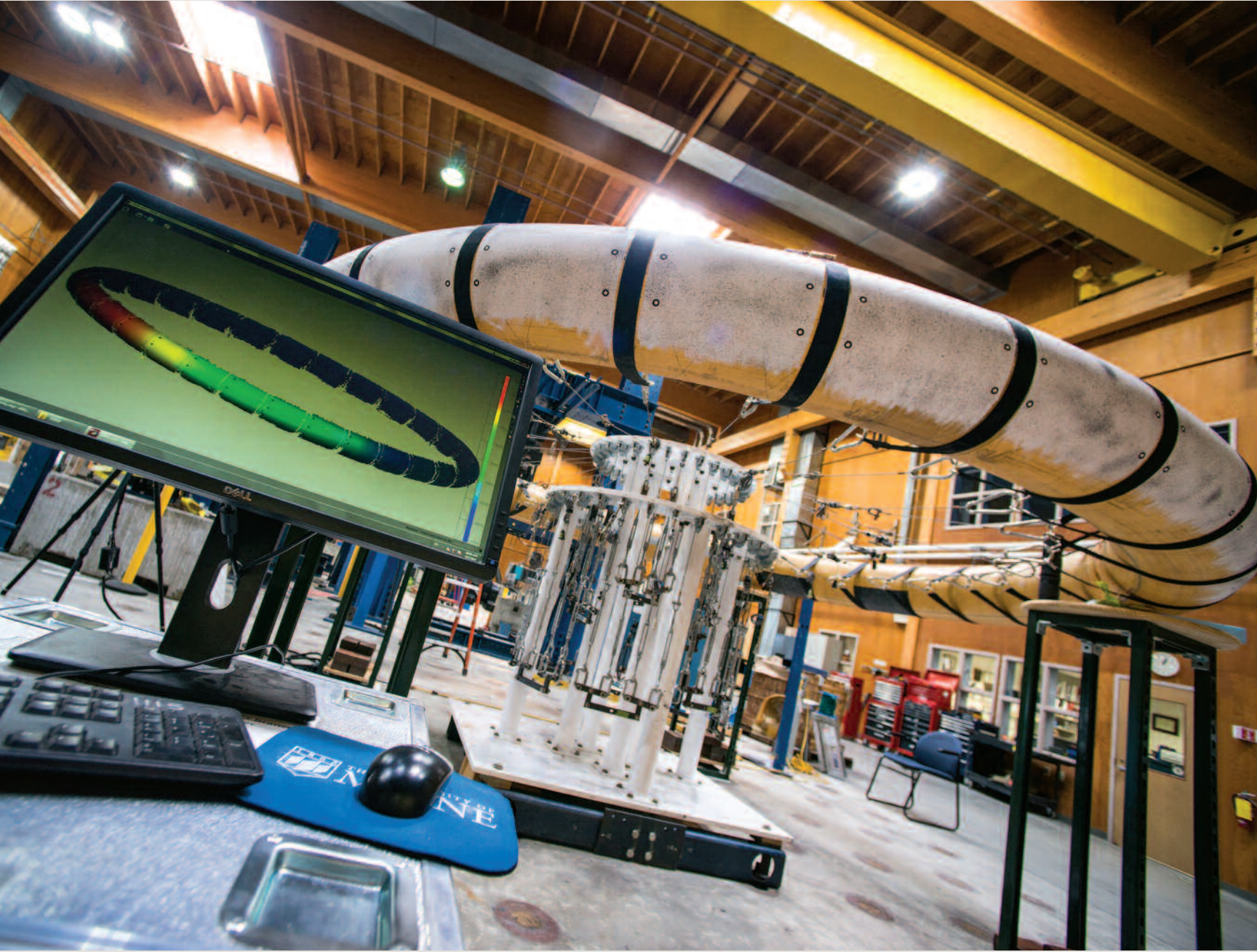
UMaine's Advanced Structures and Composites Center is collaborating with NASA to test the hypersonic inflatable aerodynamic decelerator (HIAD), designed to mount on the nose of a spacecraft and aid entry into a planet's atmosphere.
