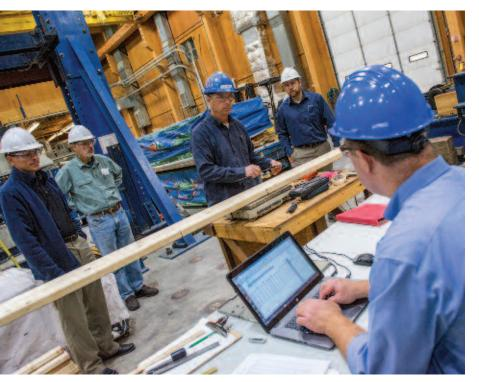
The Advanced Structures and Composites Center has an ISO 17025-accredited testing laboratory that is a valuable resource to collaborators such as the Northeastern Lumber Manufacturers Association. Norway spruce was tested to determine if it meets industry standards and can be included in the Spruce-Pine-Fir South grouping of wood species for construction-grade dimensional lumber. Preliminary results look promising, say UMaine wood scientists.
