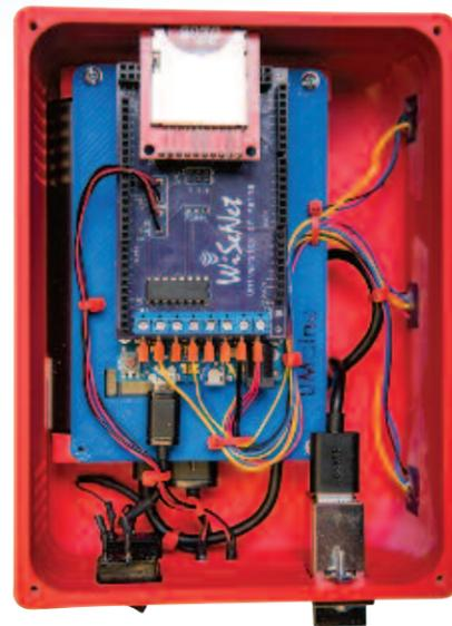
UMaine's wireless leak detection devices are expected to be ISS-bound in August. WiSe-Net Lab researchers also are exploring wireless technology with practical applications on Earth, including projects addressing issues related to veterans, aging and rural broadband.
